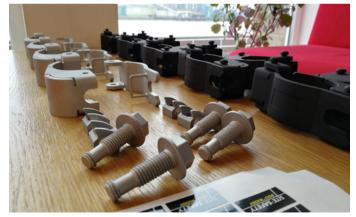
Fully functionally prototypes made from 3D printed metal.
